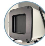
The blackbody perform as a temperature reference for accurate body temperature measurement of +/- 0.3 °C.
